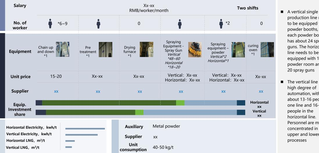
production line needs to be equipped with 2 powder booths, and each powder booth has about 24 spray guns. The horizontal line needs to be equipped with 1 powder room and 18-20 spray guns
